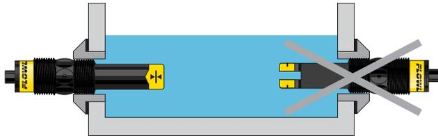
**Vibration Orientation:** Install the switch such that the forks are aligned up and down, allowing for liquid to easily leave the space between the forks. Avoid aligning the gap horizontally. This could allow material to collect on one of the forks. See the illustrations below for further information.
