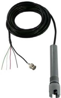
The 1520E Uses The Lakewood Instruments 520 Series Sensors For pH
