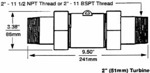
Care should be taken to adequately support and align the pipes running into and out of the turbine.
