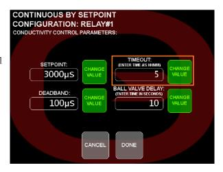
NOTE: The TIMEOUT alarm does <u>not</u> turn off the relay when using one of the BLOWDOWN options for relays 1-4 and relay 7.
