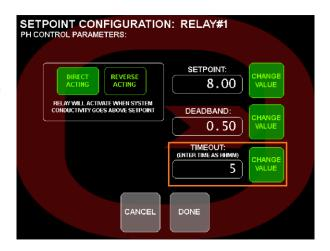
NOTE: The TIMEOUT alarm does **not** turn off the relay when using one of the BLOWDOWN options for relays 1-4 and relay 7.
