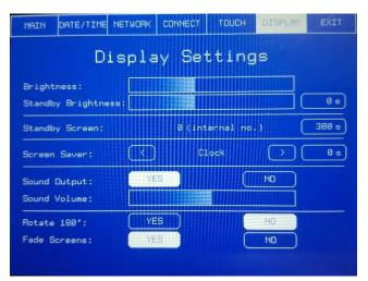
In this screen the operator can adjust the brightness of the display by touching the Brightness button. Touch on the right side of the button to increase the brightness and touch the left side of the button to decrease the brightness.
