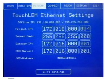
In this screen the IP settings can be changed per site requirements. This is usually only required for building automation system integration and if email notification via site intranet is required.
