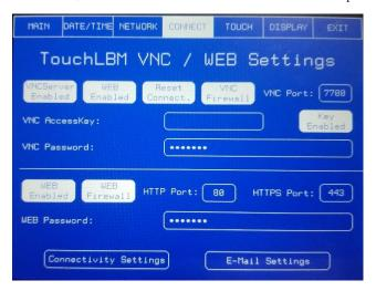
The **Remote Access Password** is set in the VNC password field. The password can be up to 16 characters long. The default remote password is PonFarr.
