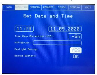
In this screen the time can be set to automatically adjust for daylight savings time and the status of the battery backup is displayed.
