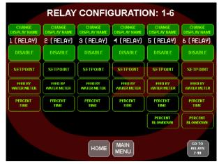
The relay configuration screen is set up to show the current configurations of the first six relays on one screen and the current configurations of relays 7 through 10 on a second screen. To switch between relays 1 through 6 and relays 7 through 10 touch the arrow buttons located at the top right of the screen.
