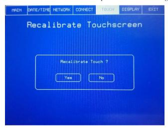
This will allow the operator to recalibrate the touch points of the display.
