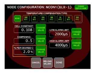
To determine that  $\alpha$  of other solutions, simply measure conductivity at a range of temperatures and graph the change in conductivity versus the change in temperature. Divide the slope of the graph by  $Gt_{cal}$  to get  $\alpha$ .
