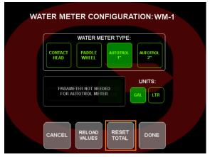
The total water meter counts can be reset to zero for each water meter input.
