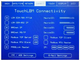
In this screen various communication protocols can be enabled or disabled and devices ID's can be changed. This is usually only required for building automation system integration via Modbus or Bacnet/IP.
