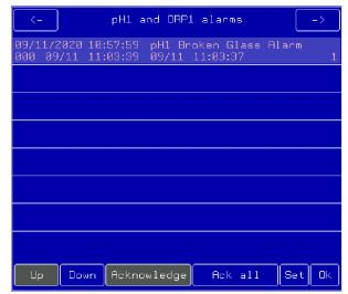
In the example above, the NexSys<sup>TM</sup> Control System logs the date and time and description of the alarm on the top line. It logs the date and time that the alarm was acknowledged and then the date and time that the alarm condition cleared on the bottom line.
