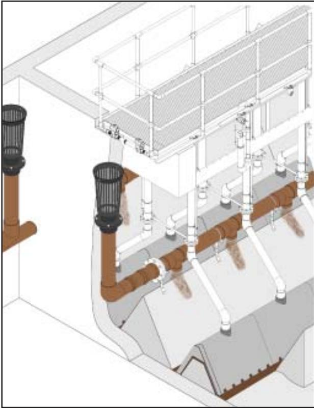
*The ClarAstor's unique effluent regulation system allows more flow to enter the plant than is exiting, creating in-basin surge storage.*
