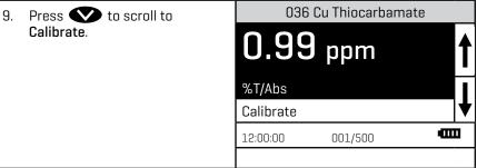
10. Press extent to select **Calibrate**. A reverse font (light background with dark characters) will appear to indicate that the reading can be adjusted.
