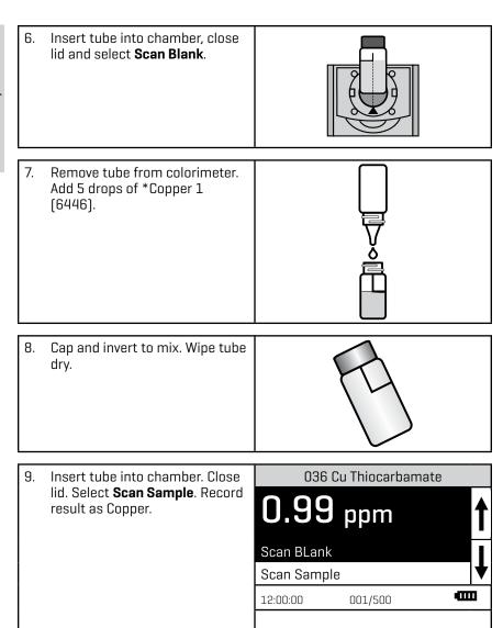
NOTE: The meter will remember the last scanned blank reading. It is not necessary to scan a blank each time the test is performed. To use the previous blank reading, instead of scanning a new one, scroll to Scan Sample and proceed. For the most accurate results, the meter should be blanked before each test and the same tube should be used for the blank and the reacted sample.
