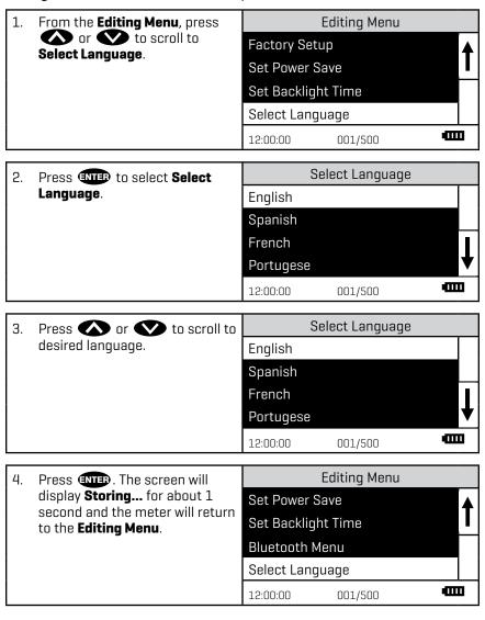
NOTE: If meter unintentionally switches to another language, use the procedure above to reset the meter to the desired language. For example, to reset the meter to English:
