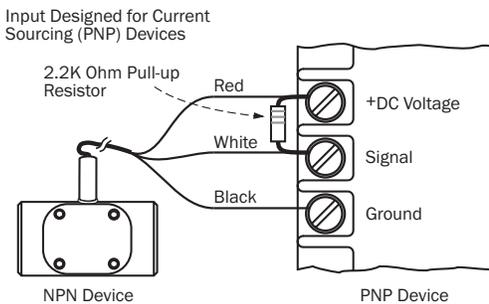
*Input designed for current sourcing (PNP) devices*
