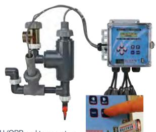
The WECT/WEDT controllers have the ability to store conductivity, pH/ORP, and temperature values, water usage, relay and flow switch status, and user settings. A USB stick is all that's needed to extract the information. Download logs from the USB stick to a PC at your convenience, or copy your preferred treatment program from another controller to speed start-up. It couldn't be easier!
