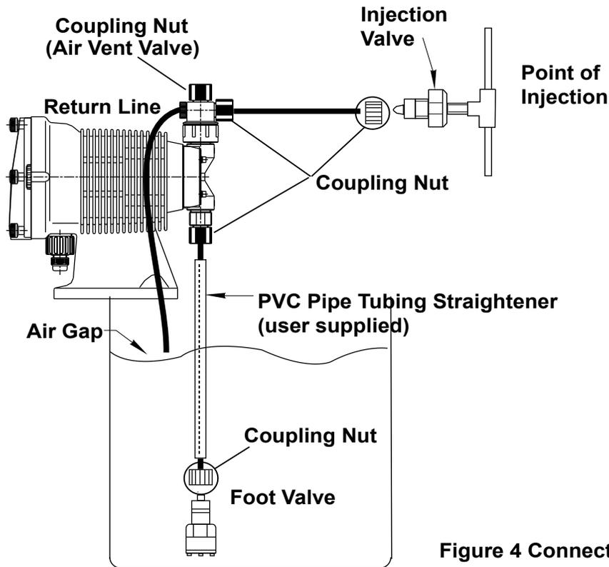
**Figure 4 Connection Tubing**
