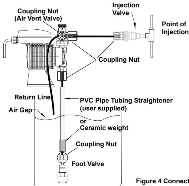
Figure 4 Connection Tubing
