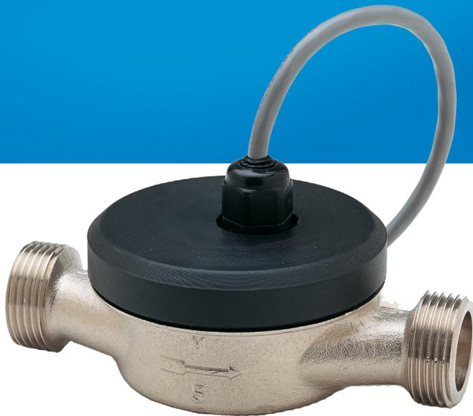
The SEB is a plated brass low flow meter suited for clean water. It is available in 1/2" and 3/4" thread, with union-type meter couplings for easy installation and service. This meter is ideal for flow rates between 0.2 GPM (0.76 LPM) and 18 GPM (68.14 LPM). The SEB has only one moving part, the propeller.
