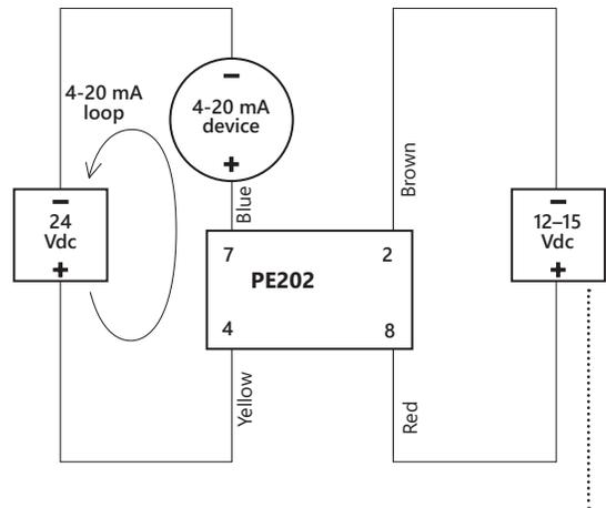
12 vdc linear power supply is recommended eg. Seametrics PC12. If dual power supply is required, please specify Seametrics PC42.
