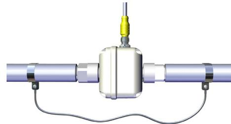
Power and signal connections are provided through the 8-pin male bulkhead connector on the meter housing (20 ft (6 m) cable provided). See the Pin Assignment and Connections diagrams.
