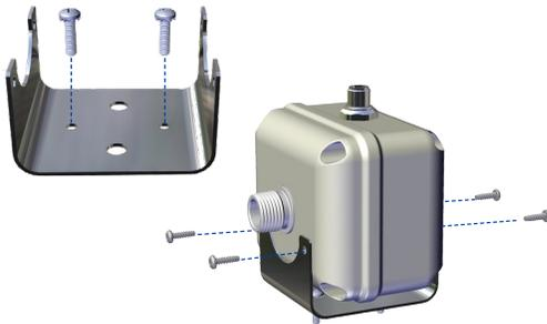
*The PE202 may be supported by its piping connections IF the piping is rigid.* The meter and pipe must be perfectly aligned with no flexion at the fittings to prevent leakage or damage to the meter.
