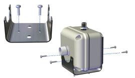
*The PE202 may be supported by its piping connections IF the piping is rigid.* The meter and pipe must be perfectly aligned with no flexion at the fittings to prevent leakage or damage to the meter.
