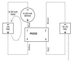
12 vdc linear power supply is recommended eg. Seametrics PC12. If dual power supply is required, please specify Seametrics PC42.
