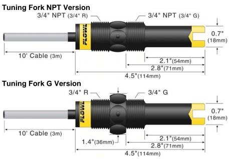
▲ The sensor should be installed so that the liquid will drip out of the gap when the sensor becomes dry.
