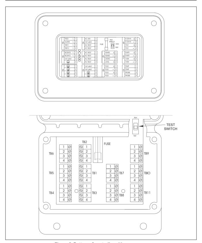
Figure 5. Bottom of controller with cover open
