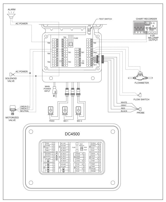
Wiring diagram for external pulse output control
