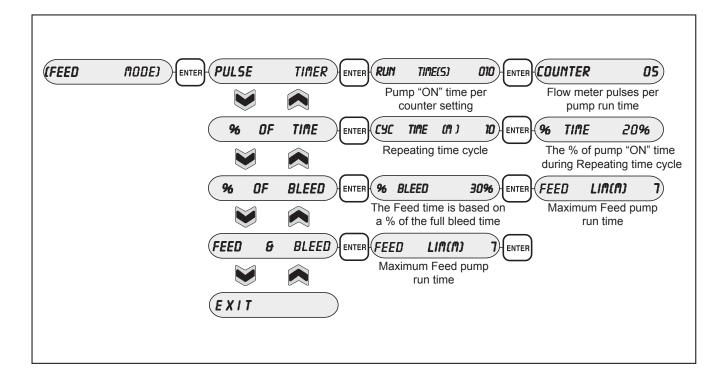
When the mode desired is displayed on the screen press "ENTER" to access the particular settings for that mode. The variables and settings that are available for each option are shown above. Use the "UP" or "DOWN" key to change the settings and press "ENTER" to save that setting.
