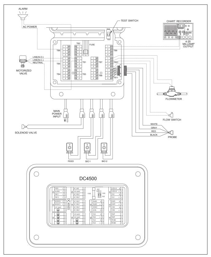
Wiring diagram for ON / OFF output control
