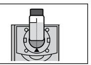
6. Remove tube from colorimeter. Add 5 drops of DPD 1A Free Chlorine Reagent (P-6740) and add 5 drops of \*DPD 1B Free Chlorine Reagent (P-6741), Cap and invert to mix. The solution will be pink if chlorine is present. Read within 30 seconds.
