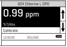
9. Press extent to select **Calibrate**. A reverse font (light background with dark characters) will appear to indicate that the reading can be adjusted.
