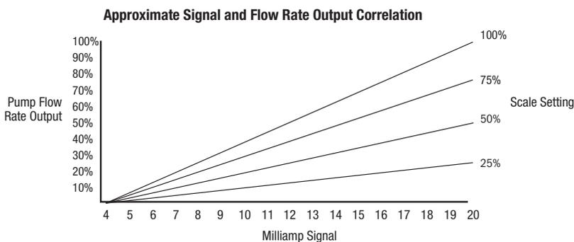
The chart illustrates the correlation between the signal received and the pump flow rate output based on the scale setting. When operating in manual mode, the adjustment range is 5% to 100%.
