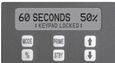
Example of control panel with keypad locked.
