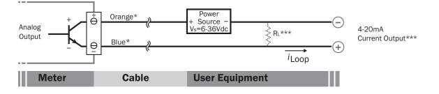
\* Wire colors shown are typical but because there are exceptions, always refer to the color codes shown on the cable label or "Control Cable Wiring" table on page 11.
