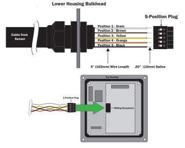
**Lengthening the Sensor Cable.** Replacing the entire cable with a longer cable is not recommended. To extend the distance from the sensor body to the remote display head: 1. Install a junction box with two holes for 5/8" connector bushings at the cable splicing location.
