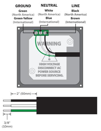
4. Tighten terminal block screws securely using 1/8" (3mm) screwdriver. Tighten the cable gland sealing nut securely. A loose nut could cause moisture ingress and compromise the meter head's IP68 rating, voiding the warranty.
