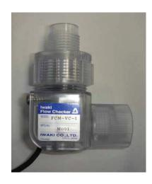
Easily mounted to the suction side of E-Series metering pumps, the FCM flow sensors use the moving liquid during the suction stroke to sense that the pump is metering chemical. With each suction stroke, liquid movement will raise a floating in-line magnet, allowing the FCM to validate flow, providing a pulse output for each verified flow pulse.
